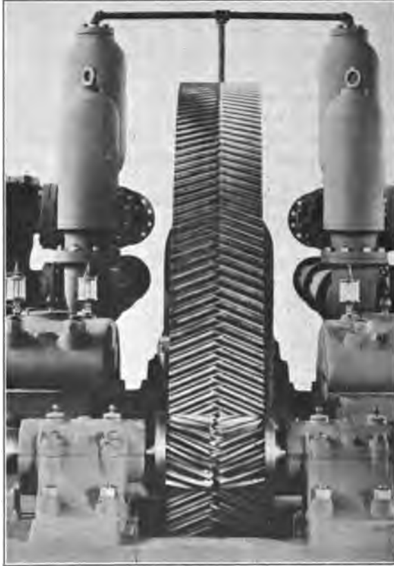
FIGURE 1. SHOWING TYPE OF HERRINGBONE GEAR REFERRED TO IN THIS PAPER.
